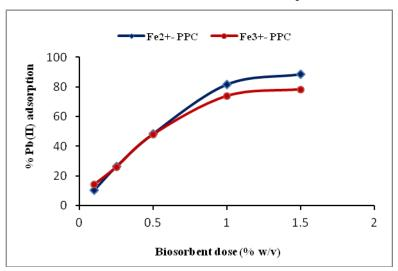
**Figure 4.** The effect of biosorbent dose on Pb(II) adsorption by iron modified pomegranate peel carbons  $(Fe^{2+}PPC \text{ and } Fe^{3+}PPC)$
