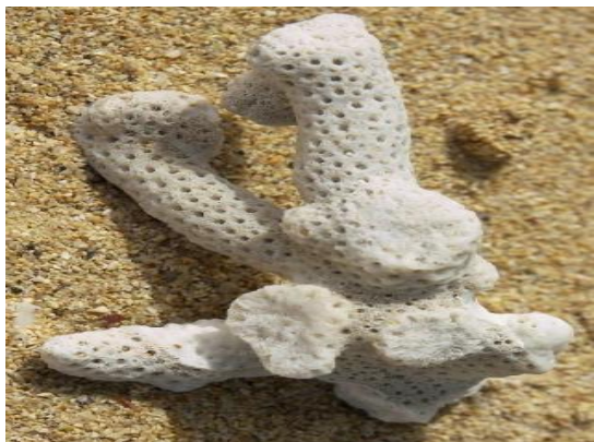
Fig. 1. The picture of the coral limestone used as sorbent
