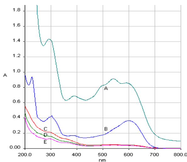
Figure 7: Absorption spectra of synthetic wastewater before and after irradiation
