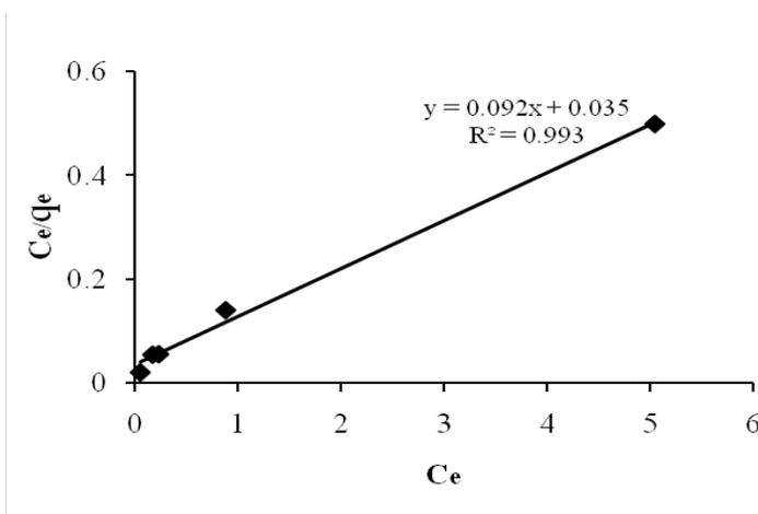
**Figure 4.** Langmuir isotherm for the adsorption of RB19 dye on different adsorbents ( $C_0=25$  mg/l, pH=7, contact time=24hr)
