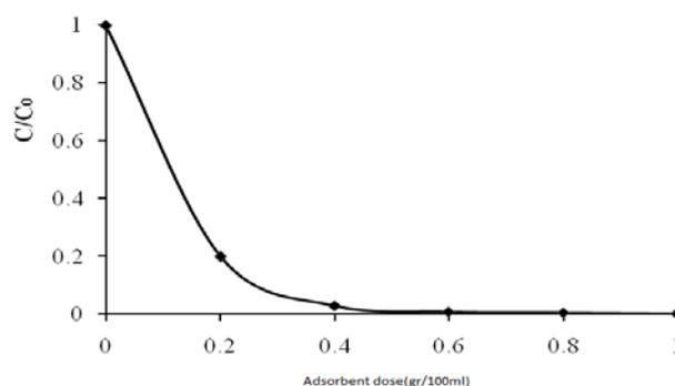
**Figure 1.** Effect of adsorbent dose on the removal of RB19 dye (dye initial concentration= 25 mg/l and pH=7)
