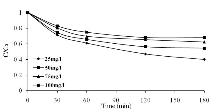
**Figure 3.** Effect of initial dye concentration and contact time on the removal of RB19 dye (adsorbent dose=0.4 gr/100ml and pH=7)
