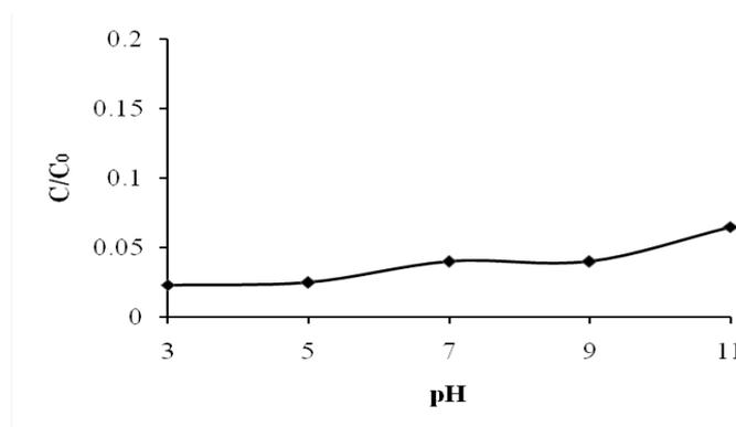
**Figure 2.** Effect of pH on the removal of RB19 dye (dye initial concentration= 25 mg/l and adsorbent dose=0.4 gr/100ml, contact time=24hr)
