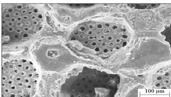
Fig. 4. SEM image of coral used as the sorbent
