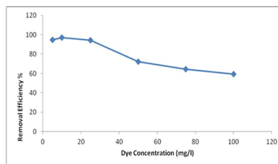
**Diagram 4.** The effect of initial concentration of the dye on dye removal efficiency (3 g of sorbent, 100 ml of dye solution, contact time of 120 min, pH=3, 25°C)
