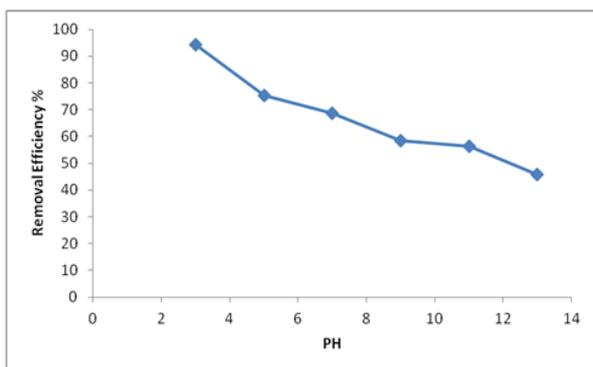
**Diagram 1.** The effect of pH on dye removal efficiency (3 g of sorbent, 100 ml of dye solution with a concentration of 25 mg/L, contact time of 120 min,  $25^\circ\text{C}$ )
