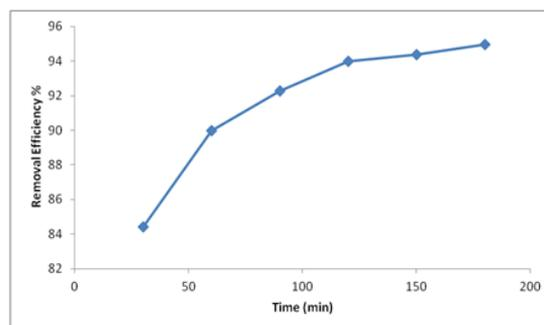
**Diagram 2.** The effect of contact time on dye removal efficiency (3 g of sorbent, 100 ml of dye solution with a concentration of 25 mg/L,  $\text{pH}=3$ ,  $25^\circ\text{C}$ )
